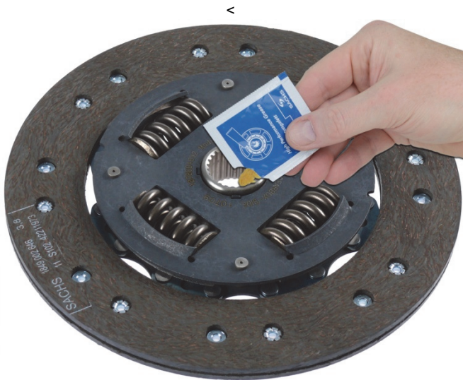
Fig.1: Lightly grease the spline hub of the clutch disc
