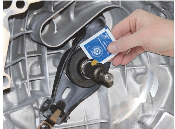
Fig. 2: Lightly grease the splines on the transmission input shaft
